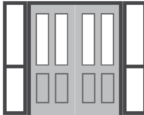
Double Doors with Glazed Sidelights and Midrails
